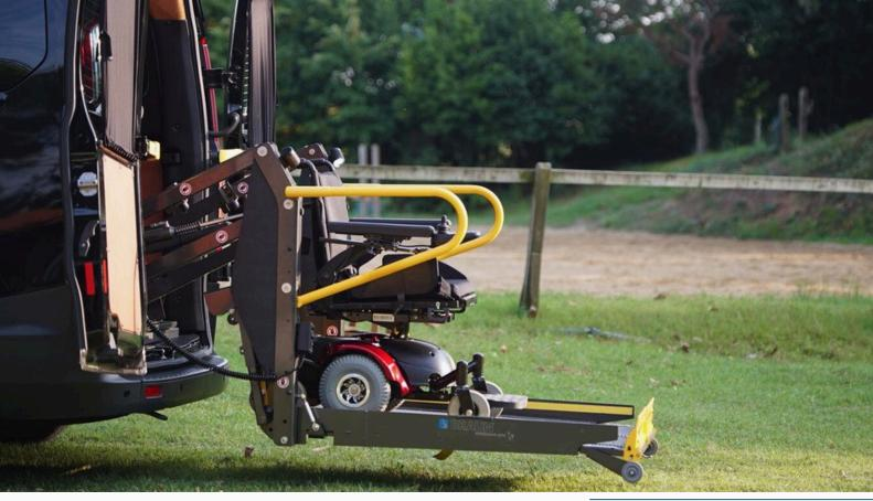
Thanks to its advanced lift mechanism, this vehicle can easily carry weights of up to **300 kg**, ensuring the safe transfer of individuals with disabilities into the vehicle.
